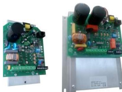
Special application inverters for AHU
